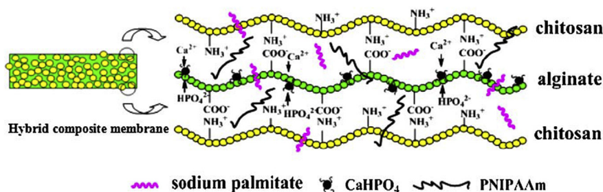
Fig. 8. Schematic illustration of hydrophobically modified alginate membrane. Reproduced with permission from Ref. [95].
